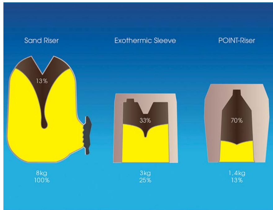
Figure 1: Comparison of sand riser/exothermic sleeve/Point-Riser
